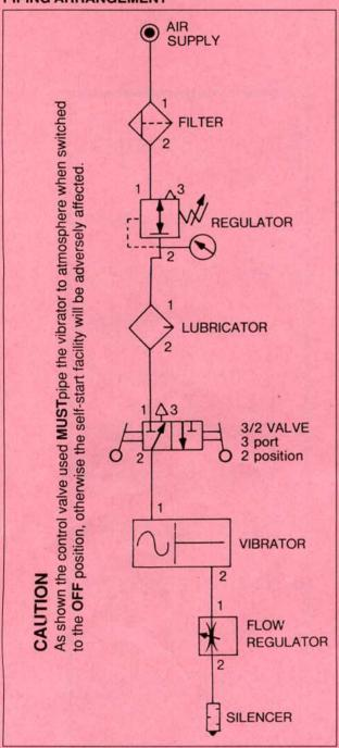
A PULSEPOWER vibrator has only one moving part, a piston, which under air pressure oscillates in a cylinder, turning at each end of its stroke on a cushion of air. The frequency of the vibrator can be altered by varying the air inlet pressure. The amplitude can be altered by restricting the air flow from the vibrator, thus creating a back pressure inside the vibrator which affects the stroke of the piston.
